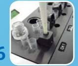
Dispense start reagent, measurement is started automatically
