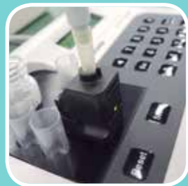
Dispense start reagent, measurement is started automatically. Result is displayed on the LCD screen or printed out automatically to an external printer
